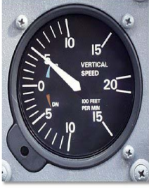
Primary for pitch when maintaining a specific rate of climb or descent
